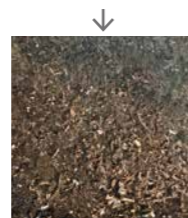
FINE FRACTION from the underflow of the SELECTOR
