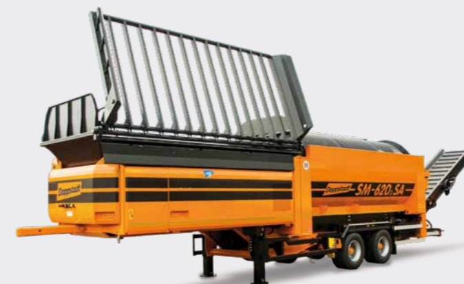
SM 620.2 SA Screening area: 30.2 m 2 Bunker volume: 7 m 3 Weight: 24,000 kg
